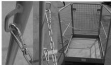
4c. Note the location of lanyard points near the floor of the basket. Use these to attach approved fall arresting devices. Also, remember to utilize the tether chain to secure the basket to the lift truck.
