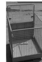
Note that this 4th hinged panel is the side that will always be closest to the mast of the lift truck, and that this panel is the tallest of the 4 when assembled
